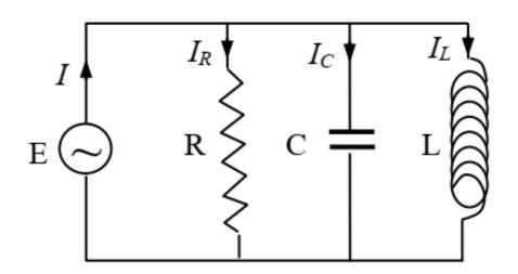
Let the branch currents through resistor, capacitor and inductor be  $I_R$ ,  $I_C$  and  $I_L$ . Let  $E = E_o \sin \omega t$  be the voltage.
