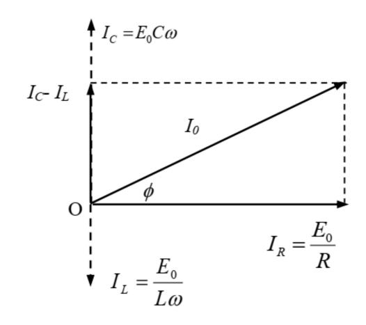
$$I = \frac{E_0 \sin \omega t}{R} + C\omega E_0 \sin \left(\omega t + \frac{\pi}{2}\right) + \frac{1}{L\omega} E_0 \sin \left(\omega t - \frac{\pi}{2}\right)$$
