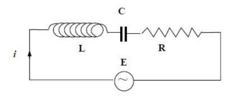
Let  $i = i_o \sin \omega t$  be the current passing through the circuit.
