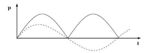
The variation of power with time over a cycle is shown in figure. Since  $V_o = I_o R$  the above relation for power can also be written as
