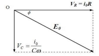
This shows that the resultant voltage lags behind the current by an angle  $\phi$
