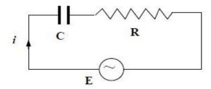
The voltage difference across the combination is E given by  $E = V_C + V_R$
