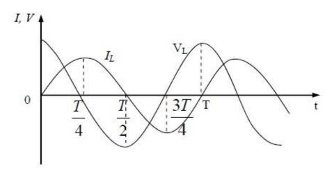
This indicates that the voltage drop  $V_L$  across the inductor is not in phase with the current.
