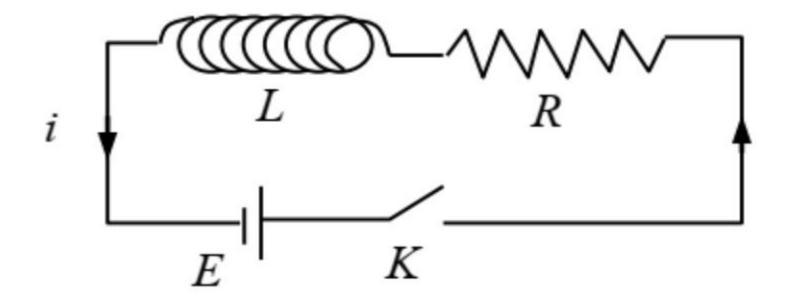
When the switch is suddenly closed, the current does not instantly rise to its final value because of the self-induced e.m.f., but grows at a rate which depends on the inductance and the resistance of the circuit.
