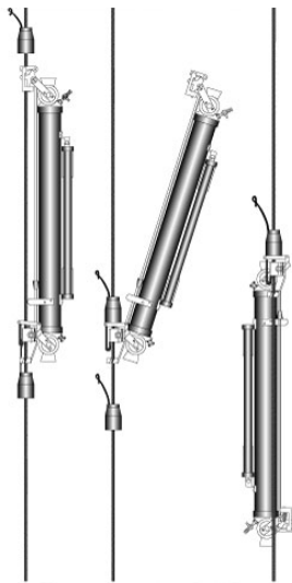
Nansen water bottles before (I), during (II), and after (III) reversing.
