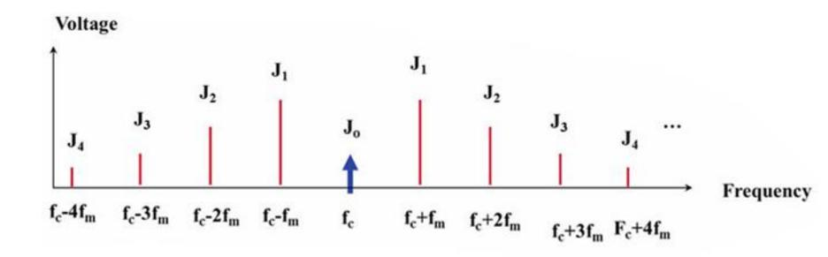
FM sidebands for large β. More power is taken from the carrier J<sub>0</sub> and distributed among the sidebands J<sub>1</sub>, J<sub>2</sub>, J<sub>3</sub>, J<sub>4</sub>,... Each sideband is separated by the modulating frequency f<sub>m</sub>
