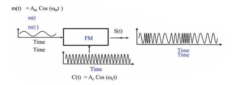
➤ A single frequency input modulating signal and its angular frequency as shown in bellow Figure. Since the frequency of the carrier varies in accordance with the input signal, the instantaneous frequency of the carrier is given by
