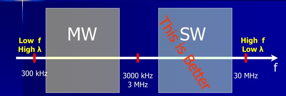
In the day time, MW is almost absorbed from the D-Region of the ionosphere. But SW are not absorbed.
