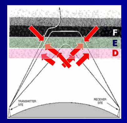
**Oscillation frequency** is the most important fact to absorb radio waves from the D-region. (Oscillation frequency is no of oscillation per second of the electrons or positive ions ) If the radio wave frequency is equal to the oscillation frequency of the D-region; the wave is absorbed from the D-region. Therefore, this oscillation frequency is the most important factor for the Radio Wave Propagation.
