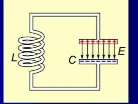
This is typically done via a **resonator** (in **the simplest form, a circuit with a capacitor and an inductor**). The resonator is configured to resonate at a particular frequency (or frequency band), thus amplifying since waves at that radio
