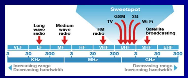
Radio **FM waves** are used because they can travel **very large distance** through the atmosphere **without** greatly **attenuated** due to scattering or **absorption**.
