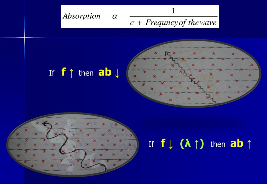
Generally, Short Waves (SW) are not much absorbed from the D-Region of the ionosphere. But, Medium Waves (MW) are normally absorbed from the ionosphere
