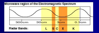
This part of the radio spectrum ranges across frequencies of roughly **1 GHz – 30 GHz**. Also by using the formula  $c = f \lambda$ , these correspond to wavelengths from **30 cm** down to **1 cm**.
