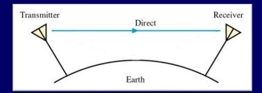
Line of sight is the **direct propagation of radio waves between antennas** that are visible to each other. This is probably the most common of the radio propagation modes **at VHF and higher frequencies**
