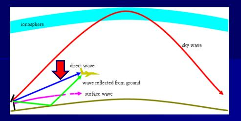
But direct ground waves also face some practical problems due to diffraction. Because the wave is bending due to diffraction. Therefore, we can not use ground waves to communicate to far.
