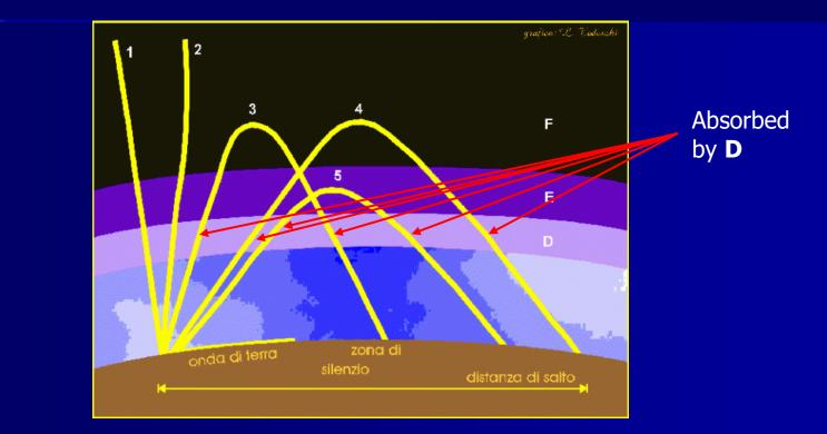
Because in the day time, radio waves reflected from the region E and F. But always the waves are going through the region D twice. (incident beam and reflected beam)
