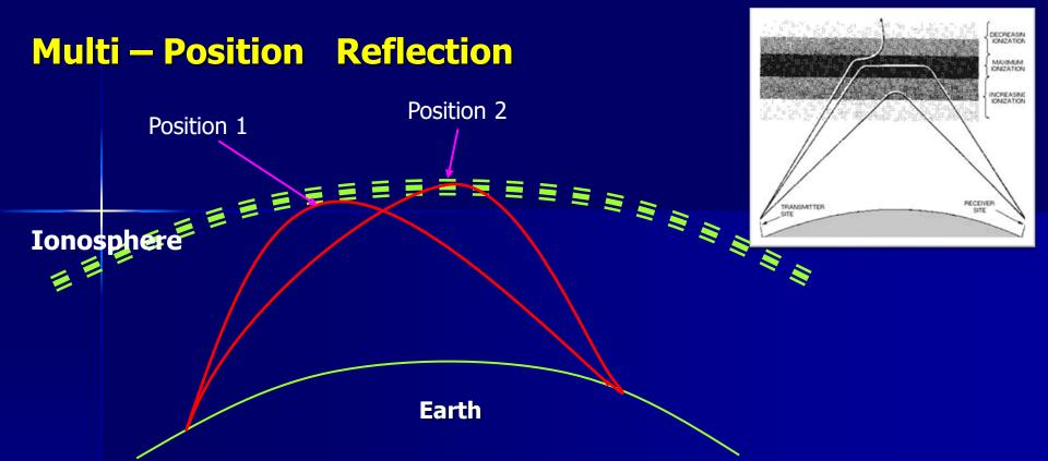
This is a possible situation. That means multi position of the ionosphere is supported to reflected the radio wave to the same receiver. **As a result the strength of the signal may be very strong**. But sometimes it may be very weak, because the **result of interference** final wave may be cancelled.
