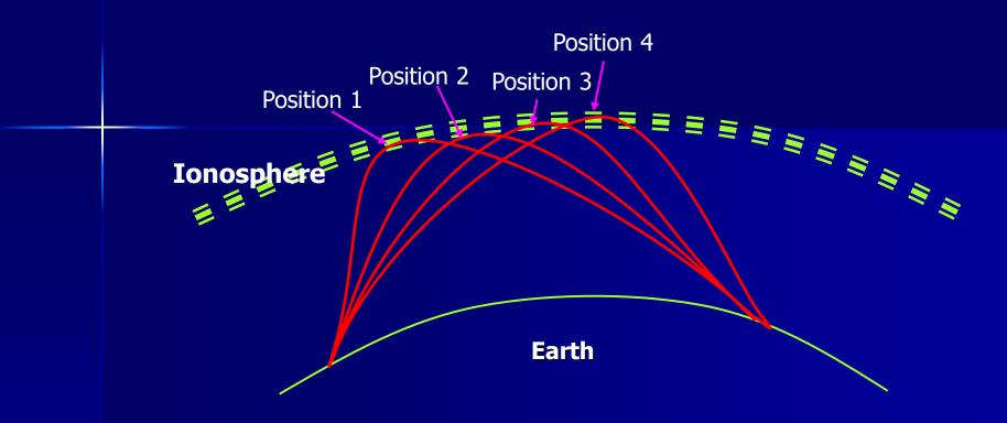
As a result of reflection of multi position final wave may be destroyed, because of the attenuation of the carrier wave of the radio signal. OR final wave may be destroyed, because of anti-phase situation (destructive interference)
