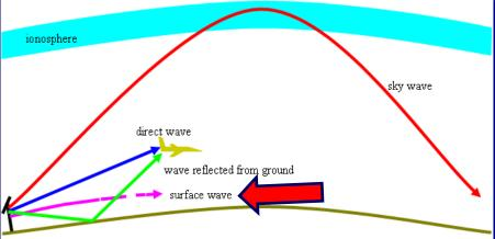
Ground waves are attenuated rapidly as they follow the Earth's surface. Attenuation is proportional to the frequency making this mode mainly useful for LF and VLF frequencies.
