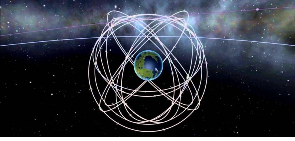
GPS is made possible by the network of 24 man-made satellites, called GPS satellites, which orbit above the Earth at great speeds and precision. Using low-powered radio waves, devices can communicate with the satellites to accurately determine one's location on the globe.
